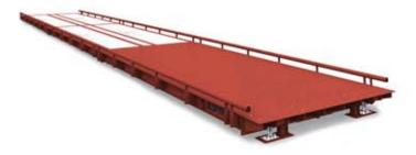
The Centurion-AT is standard with 3/8" steel or 8" concrete deck surface. Safety sight rail (shown) is an available option. The steel or concrete deck Centurion-AT weighbridge can be supplied with a hot dip galvanized finish for extreme corrosion protection.
